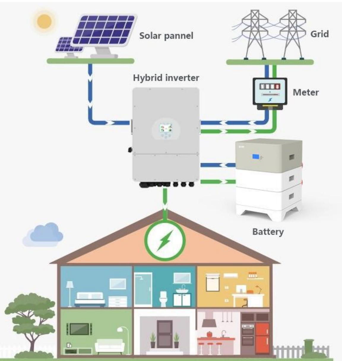
Micro-Grid is composed of a small power distribution system consisting of distributed power sources, Solar power system, energy storage batteries, energy conversion devices, load, monitoring and connection and protection devices.
